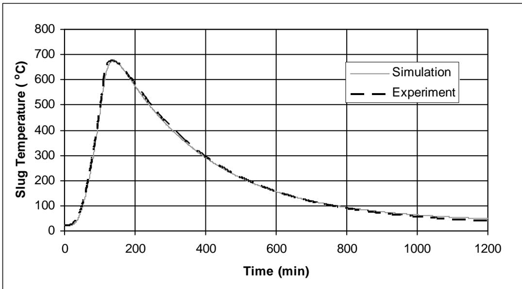
Figure 8. Experimental and model predicted exterior FRM surface (top) and slug temperatures (bottom) vs. time for the second heating/cooling cycle in the slug calorimeter for the medium density FRM.
