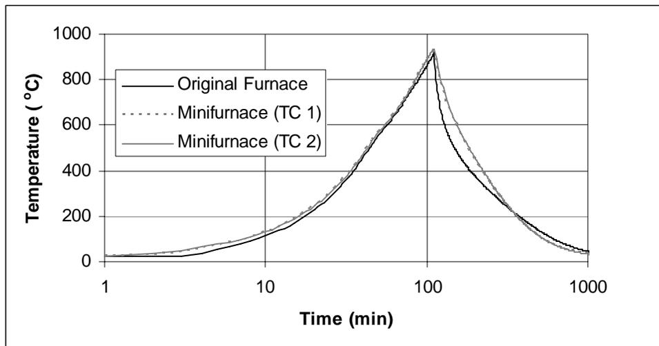
**Figure 2. Comparison of measured furnace temperatures for the original furnace and the mini-furnace when programmed with the same set of linear temperature ramps. TC1 and TC2 indicate two different locations of sensing thermocouple in the mini-furnace as described in the text.**
