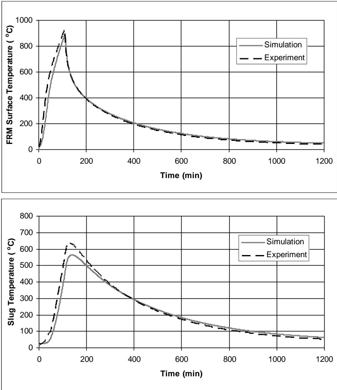
**Figure 10. Experimental and model predicted exterior FRM surface (top) and slug temperatures (bottom) vs. time for the first heating/cooling cycle in the slug calorimeter in the original furnace for a standard density (specific gravity = 0.31) FRM.**
