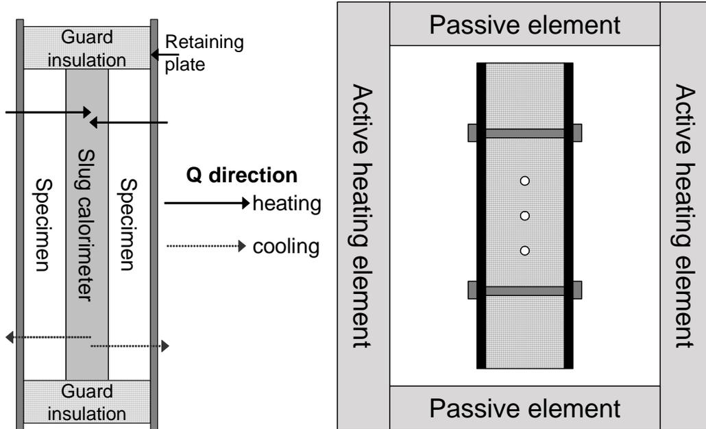
**Figure 1. Schematics of the slug calorimeter test setup: left- schematic of a cross section through the middle of the basic slug calorimeter setup, and right- schematic of an overhead view of a completed sandwich specimen mounted and ready for testing in the mini-furnace.**
