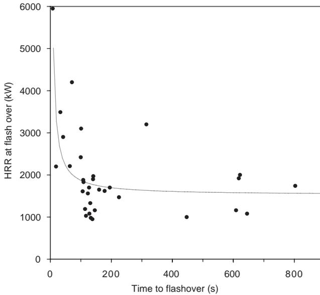
Fig. 2. Effect of time to flashover on the HRR required for flashover.
