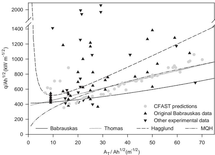
Fig. 3. Comparison of predictions of minimum flashover energy with additional real-scale fires for a range of compartment and opening sizes.
