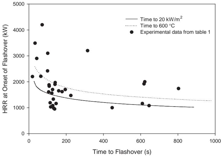
Fig. 4. Predicted HRR at flashover for  $t^2$  fires with a range of characteristic fire-growth rates, compared to experimental data.
