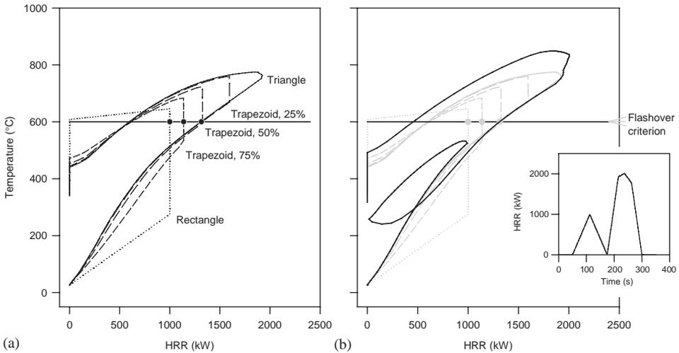
Fig. 5. Effect of the shape of the HRR curve on the upper layer temperature for a single compartment scenario.
