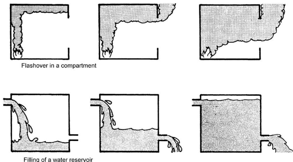
Fig. 1. Flashover as a room-filling process, and analogy to a water reservoir [7].
