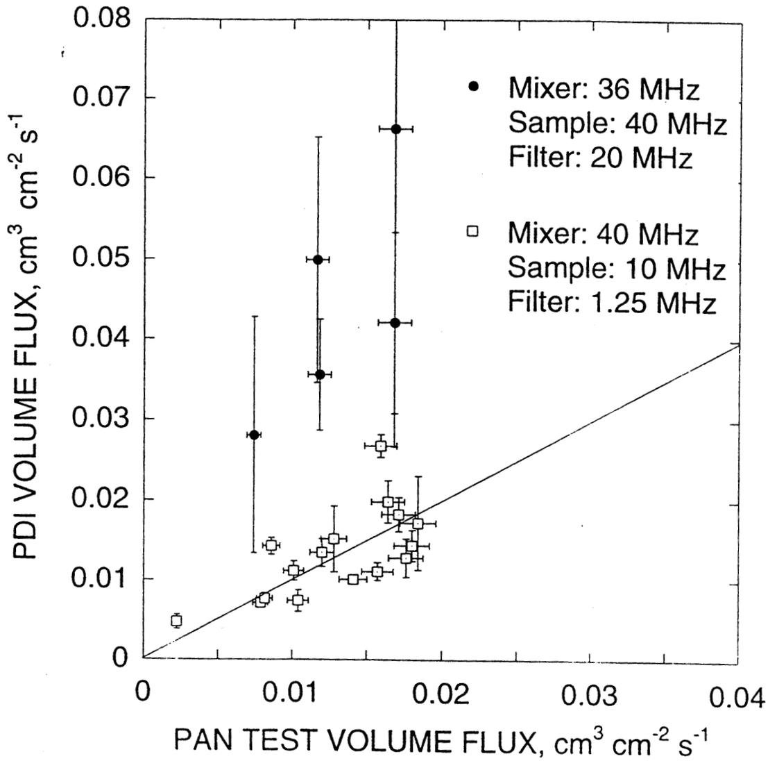
Fig. 11 Comparison of the volume flux measured with the PDI system and the pan test measurements.
