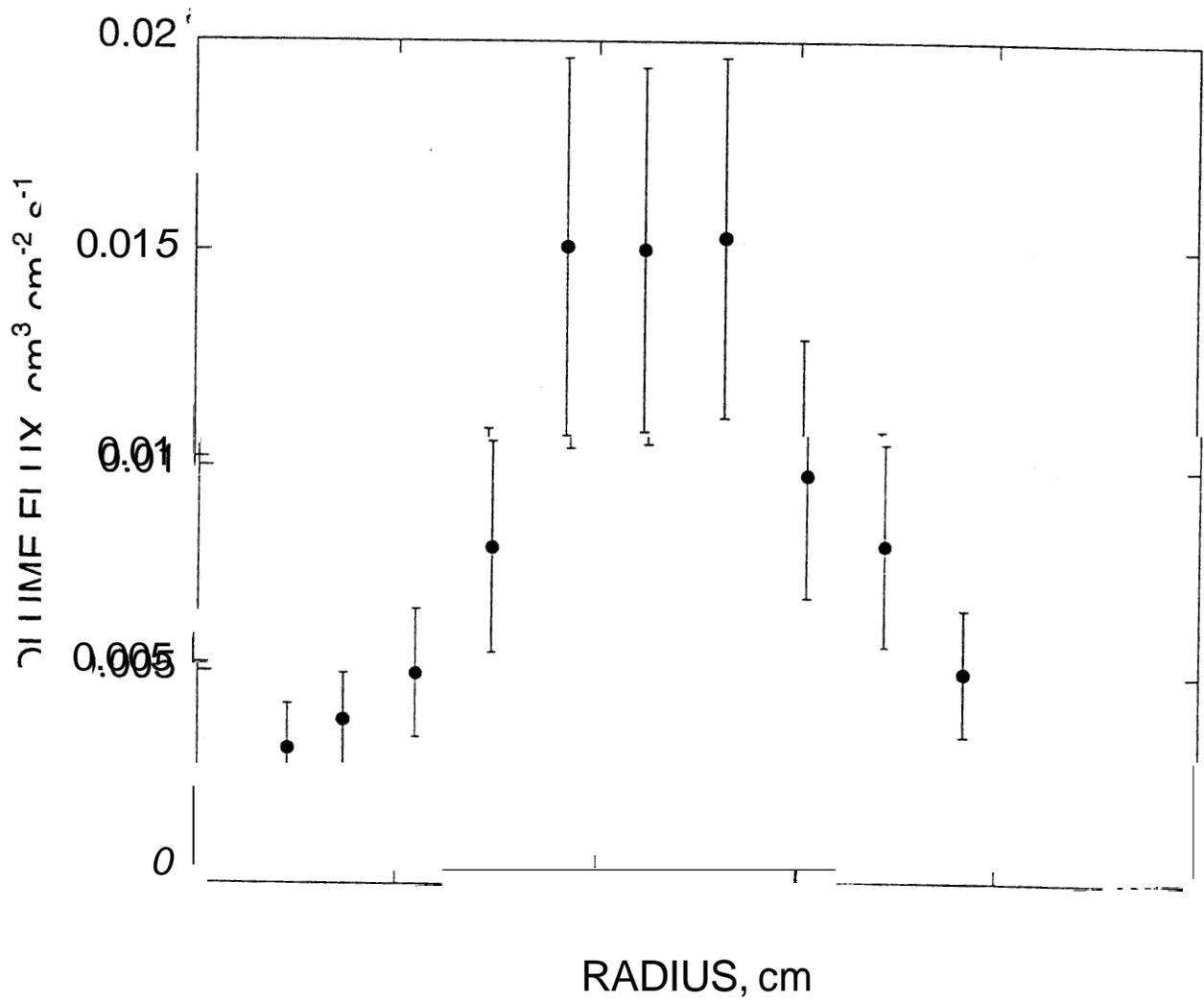
Fig. 6 The volume **flux** measured with the PDI system as a function of the radial coordinate.
