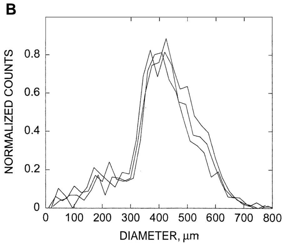
Fig. 3 Representative size distributions obtained with the PDI system at locations (A) near and (B) far from the fire sprinkler axis.
