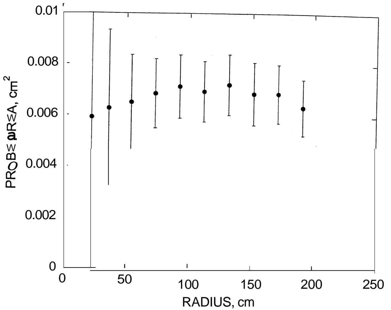
Fig. 13 The measured probe area as a function of the radial coordinate.
