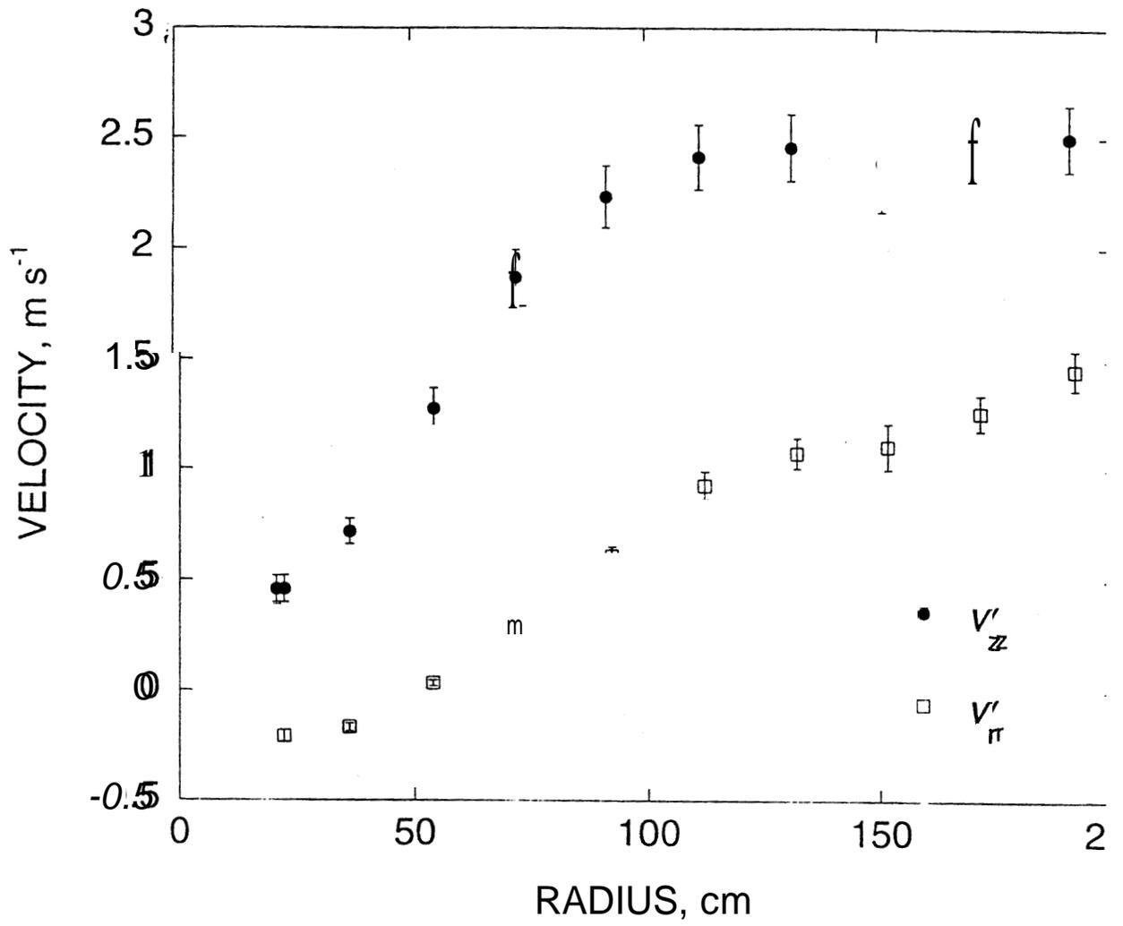
Fig. 5 The mean axial and radial drop velocities measured in the spray as a function of the radial coordinate.
