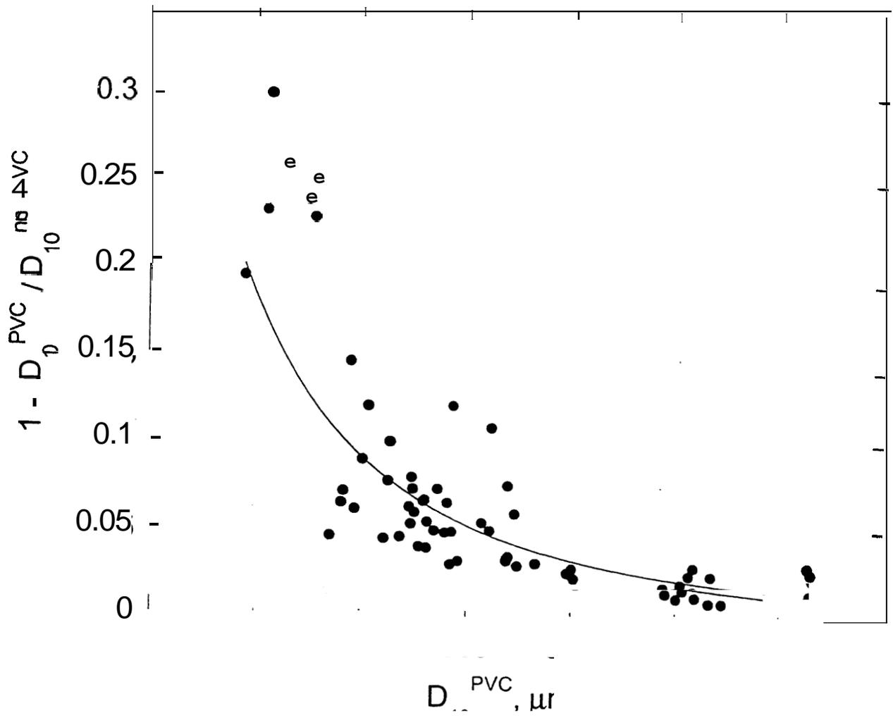
Fig. 8 The effect of the probe volume correction on the arithmetic mean diameter,  $D_{10}$ .
