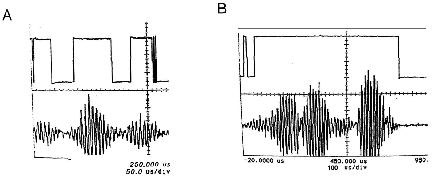
Fig. 12 Oscilloscope traces showing the effect of burst splitting on the gate signal and the Doppler signal. The operating conditions correspond to (A) mixer frequency = **36 MHz**, sample frequency = **40 MHz**, and low pass filter = **20 MHz**, and (B) mixer frequency = **40 MHz**, sample frequency = **10 MHz**, and low pass filter = **1.25 MHz**.
