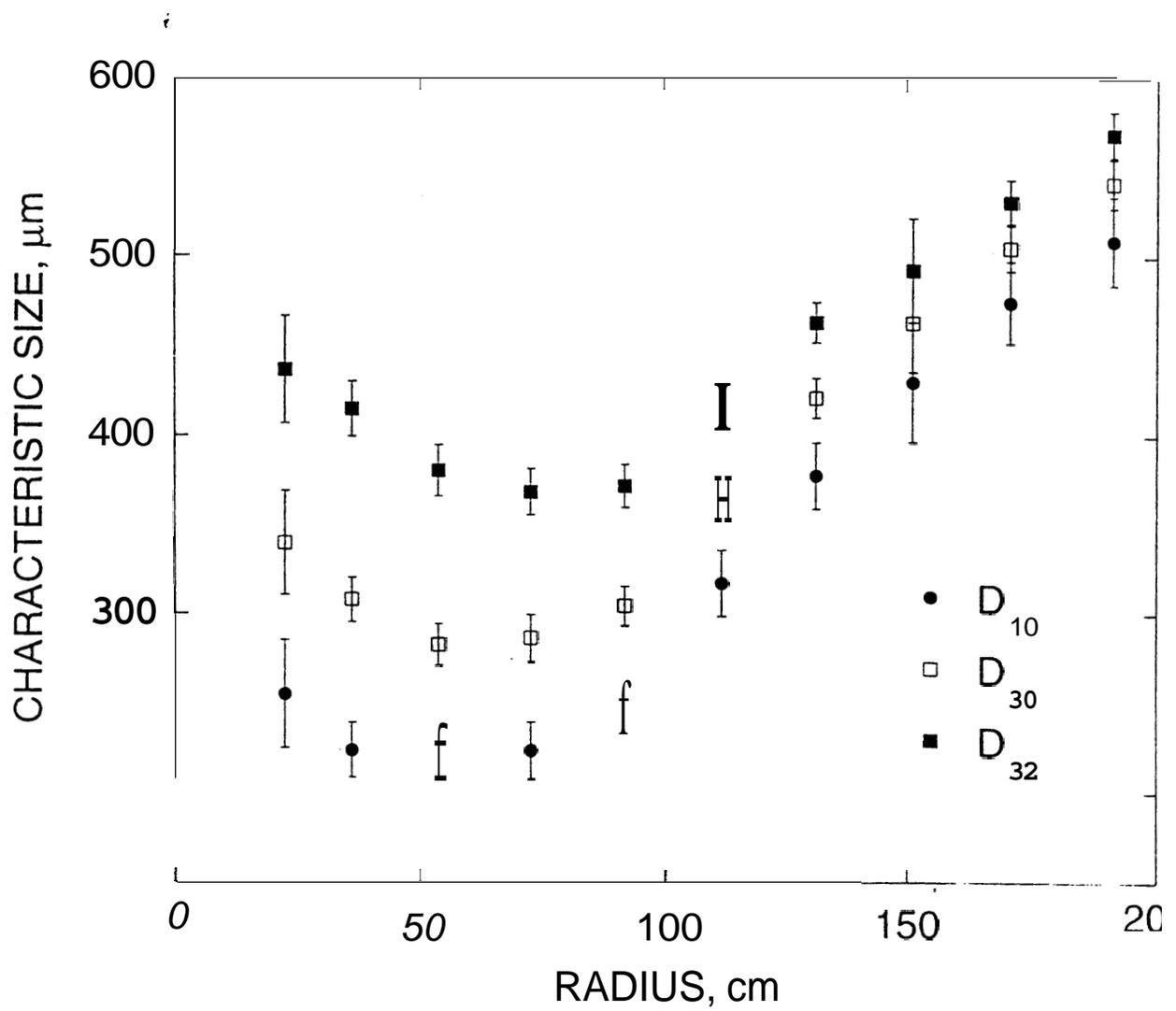
Fig. 4 The arithmetic mean diameter ( $D_{10}$ ), volume mean diameter ( $D_{30}$ ), and Sauter mean diameter ( $D_{32}$ ) as a function of the radial coordinate in the spray.
