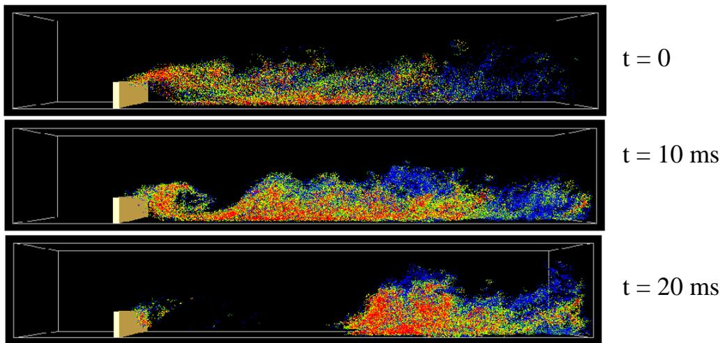
Propane flame extinction behind 25 mm baffle with 100 ms  $N_2$  pulse.
